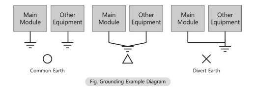
(4) Keep ground near the instrument and keep the ground wire as short as possible.
