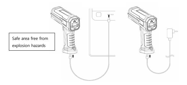
O Do not charge the battery or connect a data cable in explosive areas.
